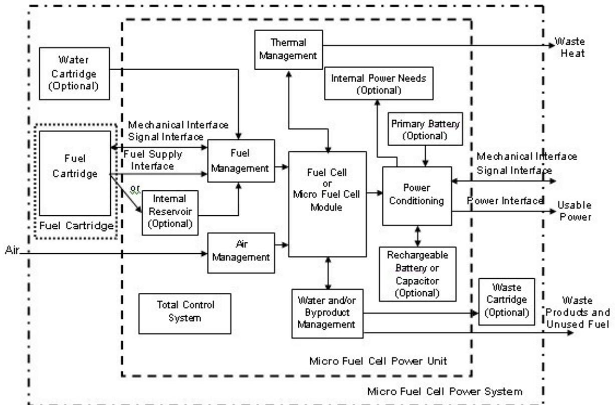
Figure 1 – Micro fuel cell power system block diagram
