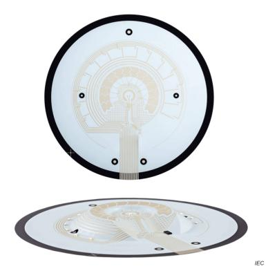
NOTE 1 The top image shows a 2D substrate and ink stack after printing and cure.
