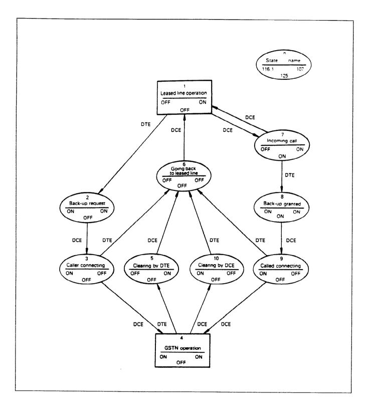
Figure 1 — Back-up Switching in "Direct Mode"
